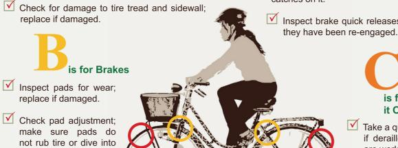
is for Check it Over ▼ Take a quick ride to check if derailleurs and brakes are working properly.
